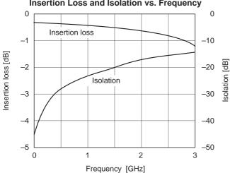
Insertion Loss and Isolation vs. Frequency
