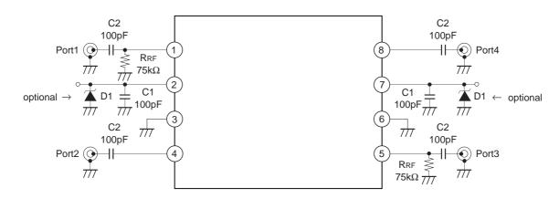
When using the CXG1017N, the following external components should be used:
