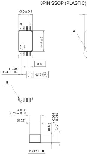
NOTE: Dimension "\*" does not include mold protrusion.
